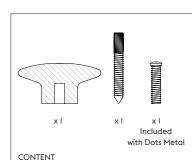
1. Before mounting your Dot to the wall, drill a 6 mm hole and add a plug.
